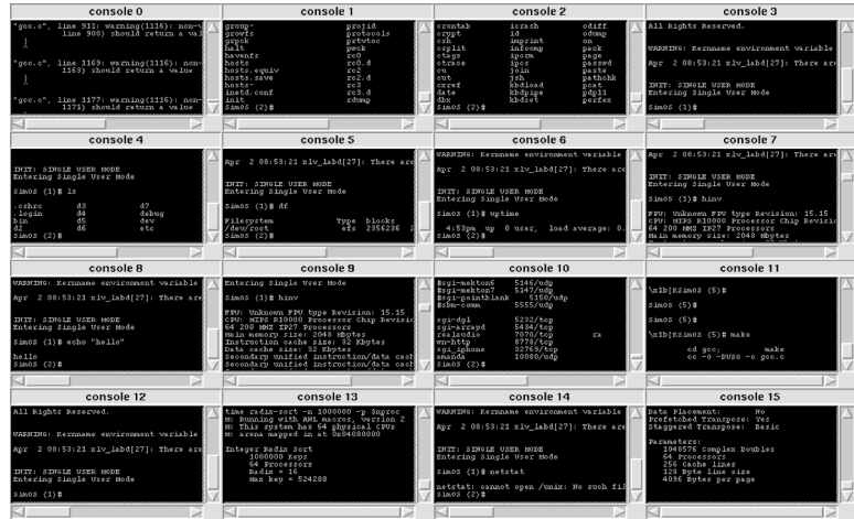
Figure 6: 1024-processor System Boot. Exploring the limits of resource overcommitment (1024 virtual CPUs on 8 real CPUs) for interactive use, our Tcl/Tk-based console tool displays a simulated cluster of 16 64-processor machines running 8-way parallel. Varying programs and activities appear in different panes of the virtual console tool.
