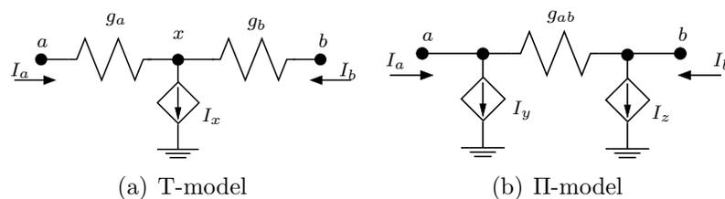
Figure 2.4: Converting a T-model to a  $\Pi$ -model.
