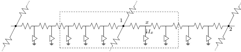
Figure 2.2: Schematic of the detailed extracted power grid of Figure 2.1.
