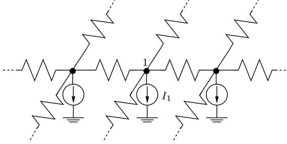
Figure 2.3: Schematic of the simplified extracted power grid of Figure 2.1.
